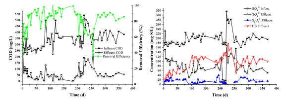
**Figure 1.** Performance of the SRUSB reactor. (a) influent and effluent COD concentrations and COD removal efficiency; and (b) influent and effluent sulfate concentrations, effluent sulfide and thiosulfate concentrations
