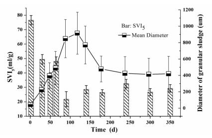
**Figure 2.** Particle size distribution and  $SVI_5$  of the sludge during granulation. Boxes and whisker plots are the mean and standard deviation values of the particle size distribution while the columns are  $SVI_5$  values.
