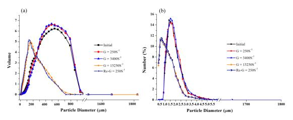
**Figure 3** Behaviour of SRB granules when subjected to the cohesion test: (a) PSD by volume and (b) PSD by number.
